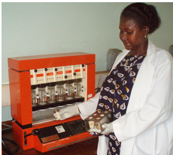
Margareth Kibodya collecting data, detemining fat content of tilapia feed containing proteins from local plants in Tanzania. (Courtesy of Kwamena Quagrainie)
